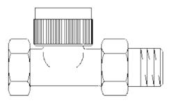
TRV "Series AZ" with high kv value straight pattern valve, DN20 - 3/4"
