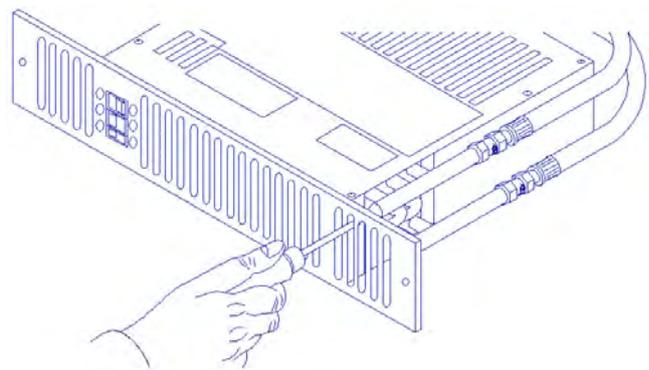
4. Isolate electrical supply and connect the heater electric cable to the fused spur (5A). Ensure the fused spur is not directly above the heater and is accessible after installation is complete.
