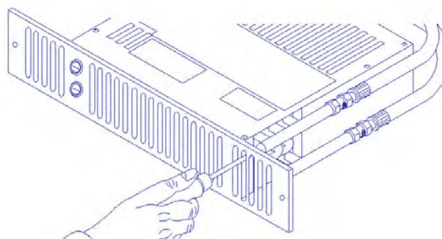
4. Isolate electrical supply and connect the heater electric cable to the fused spur (3A). Ensure the fused spur is not directly above the heater and is accessible after installation is complete.
